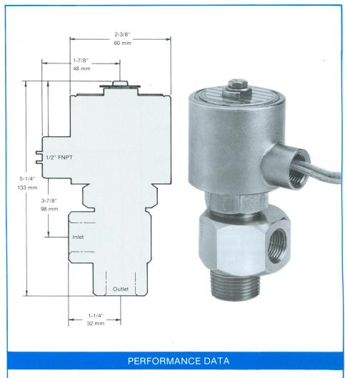
Voltage: AC as specified Fluid: Liquid carbon dioxide (CO<sub>2</sub>) Operation pressure: 3-350 psig Rated pressure: 350 psig Flow factor (CV): 3
